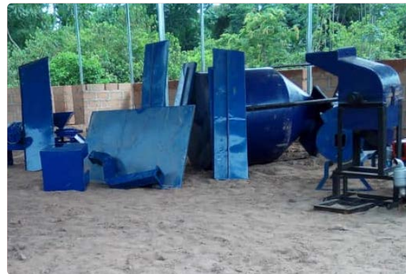
Palm kernel extractor in process of being mounted
